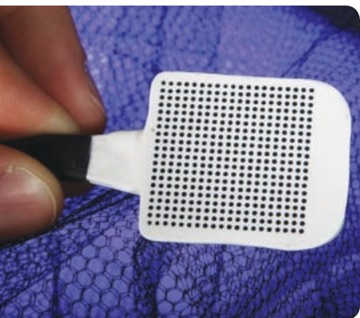
"LOLLIPOP" DEVICE is an electrode array that stimulates the tongue in a pattern based on the light intensity picked up by a camera.
