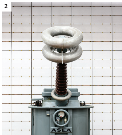
Holbøll with a high-voltage sphere gap (1). A 400,000-volt single-phase transformer (2).
